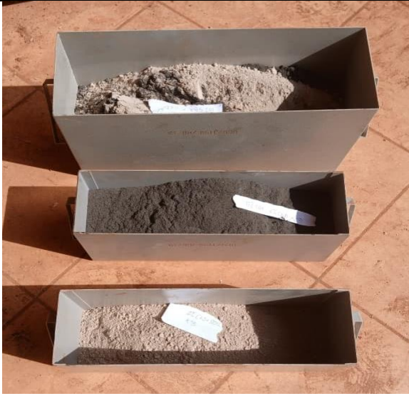
Figure 8: An image of the soil, SBA, and CKD in batching portions.
