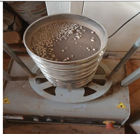
Figure 10: An image of the Particle Size Distribution test
