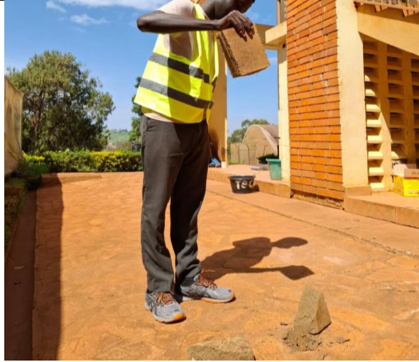
Figure 12: An image of the block drop test in progress
