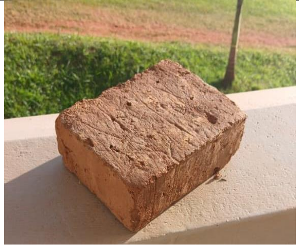
Figure 13: An image of the final brick product with 10% SBA & 6% CKD
