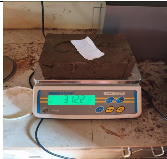
Figure 11: An image of a brick sample with 20% SBA & 6% CKD being weighed
