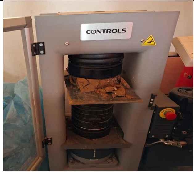
Figure 9: An image of the compression test on brick samples
