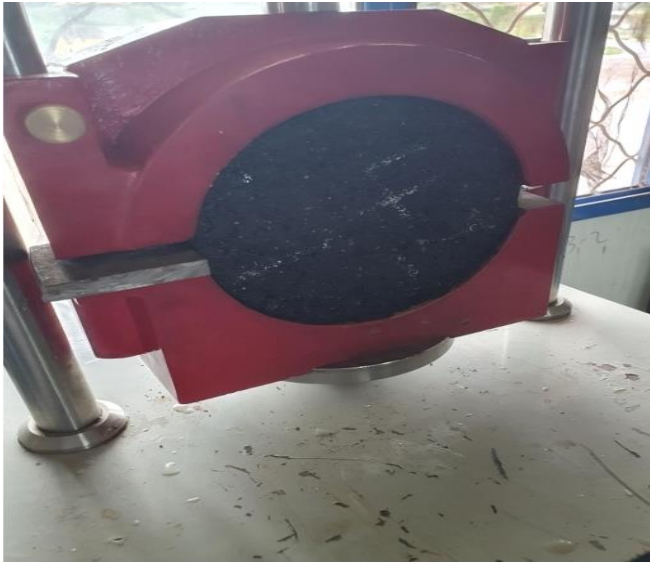
Appendix 1: Marshall Flow and Stability Testing
