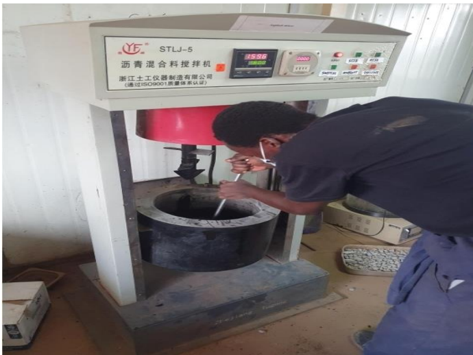
Appendix 2: Mixing of Bitumen and aggregates for Marshall Compaction
