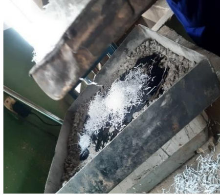
Heating and Melting Polypropylene in Bitumen
