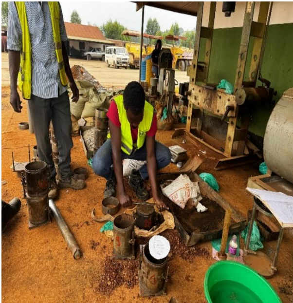
Figure 14 Preparation of CBR mold
