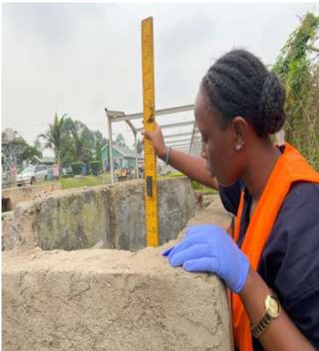
Figure 27: Sludge depth measurement
