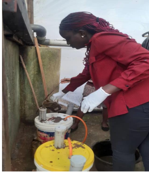
Figure 13: feeding of digesters
