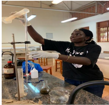
Figure 2: Titration of sulphuric acid during FOS/TAC test
