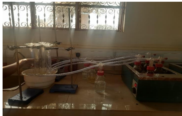
Figure 5: BMP test set up
