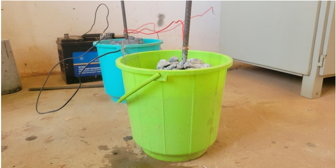
Figure 6: Showing accelerated corrosion test set up
