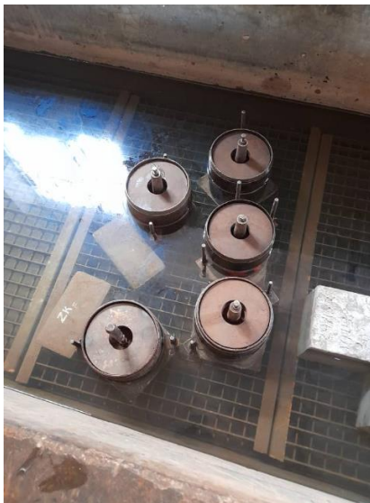
Figure 22: Shows moulds soaking
