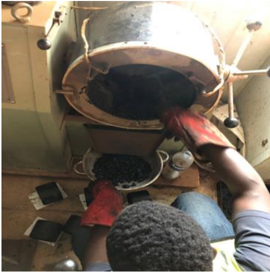
Figure 17: Showing Drum mixer for Asphalt Hot Mix.
