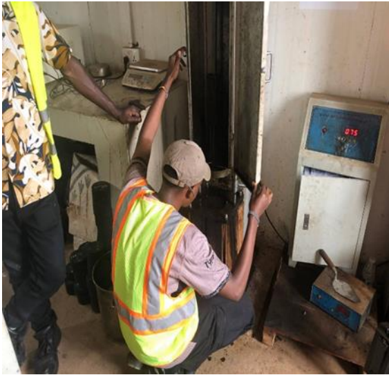
Figure 13: Showing Operation of a Marshall compactor.
