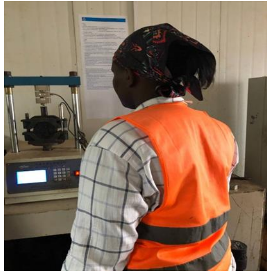
Figure 14: Showing the reading the Stability Test Results.
