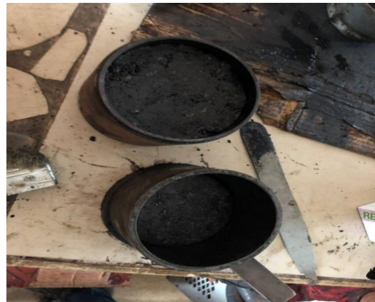
Figure 16: Showing Sample Molds of Modified Asphalt Concrete
