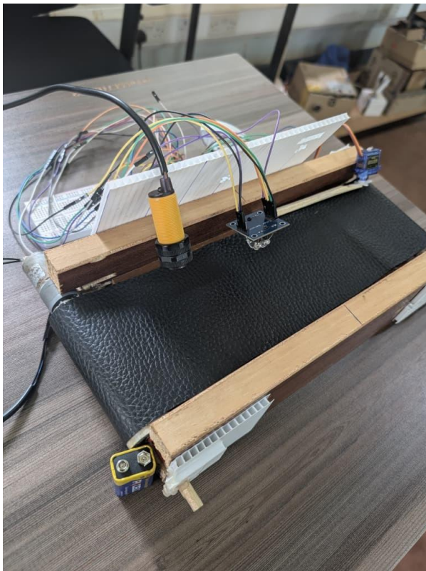
(a) Conveyor belt texture and sensors
