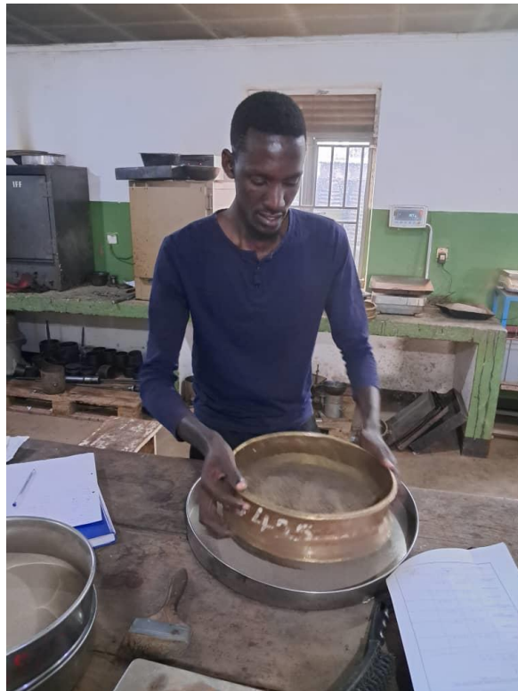
Figure 2: Carrying out a particle size distribution test
