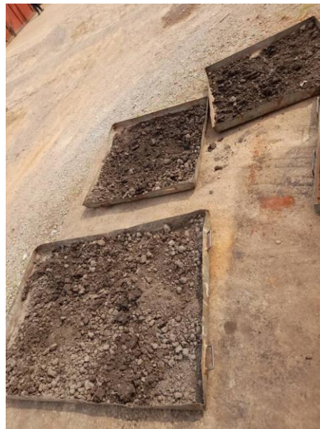
Figure 1: Drying a neat sample of the weak soils.
