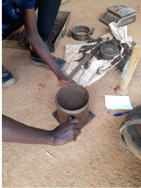
Figure 3: Carrying out a proctor compaction test
