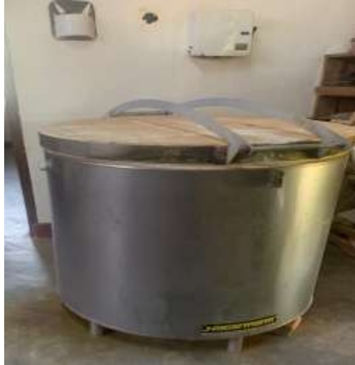
Figure 5: The electric kiln used in processing the activated press mud
