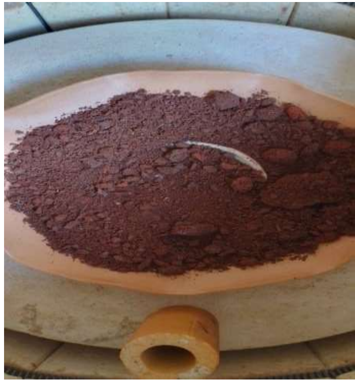
Figure 3 Activated press mud in the electric kiln
