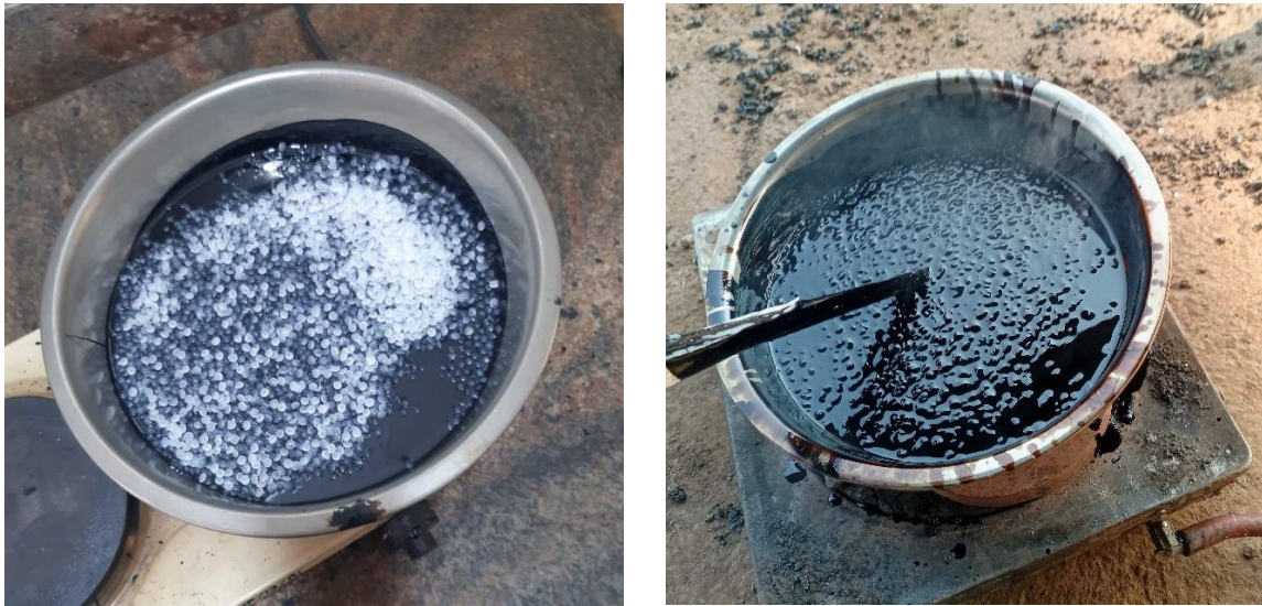
Figure 14: LLDPE mixed in molten bitumen to acquire homogenous mix
