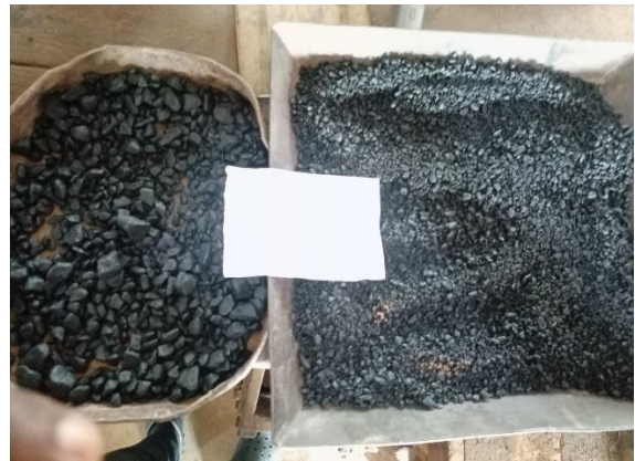
Un-compacted asphalt mixture for Gmm
