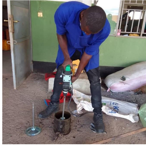
Compacting specimen to refusal density
