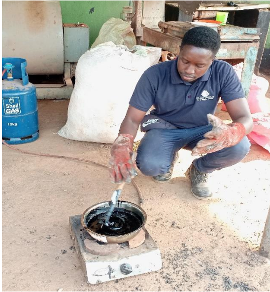
Mixing bitumen and LLDPE homogenously
