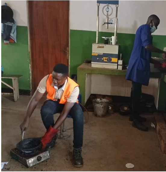
Mixing aggregates and bitumen
