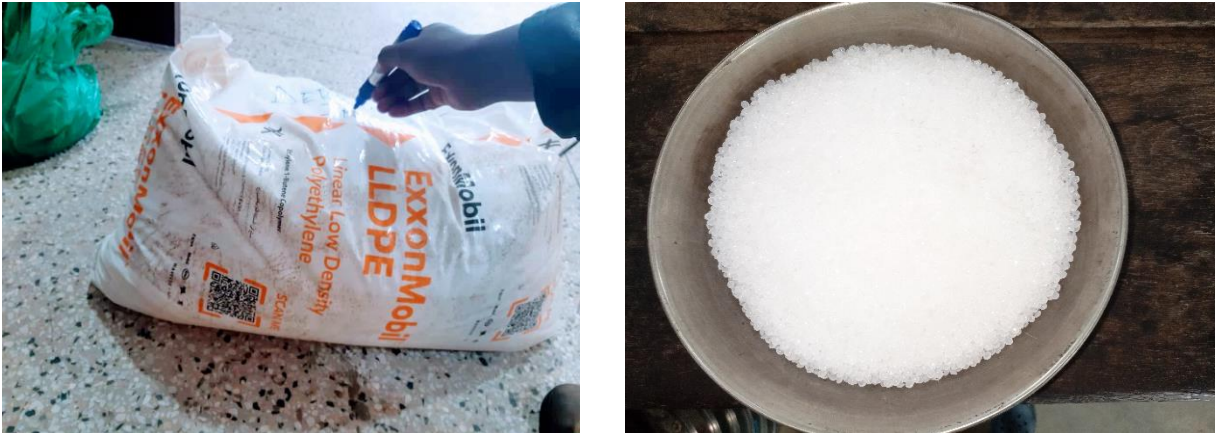
Figure 13: Linear-Low Density Polyethylene used for bitumen modification
