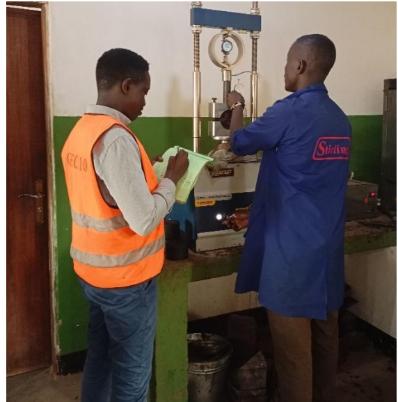
Conducting Marshall stability and flow test
