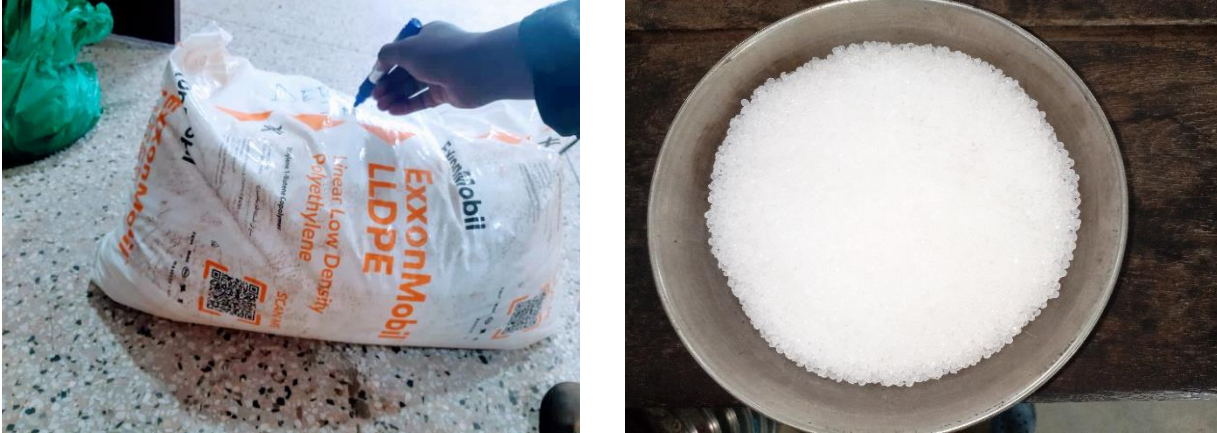
Figure 14: Linear-Low Density Polyethylene used for bitumen modification
