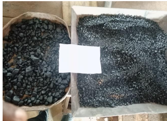
Un-compacted asphalt mixture for Gmm
