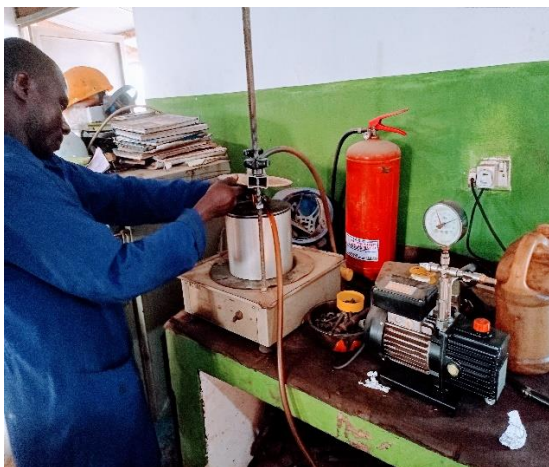
Testing for maximum specific gravity of asphalt mixture
