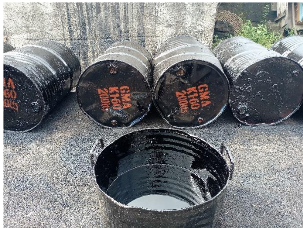
Figure 13: Acquiring bitumen sample
