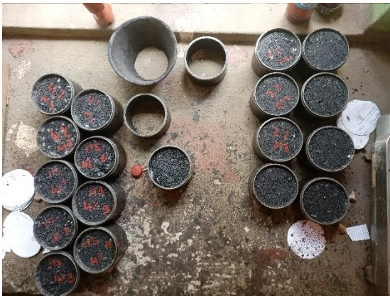
Compacted asphalt specimen
