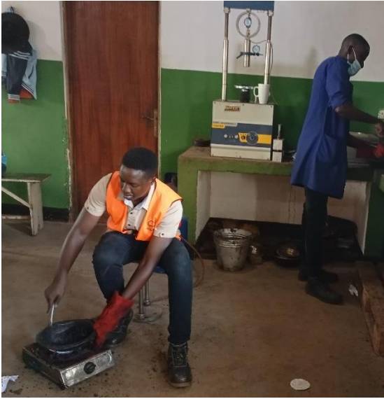
Mixing aggregates and bitumen
