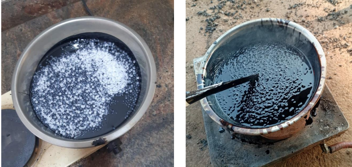
Figure 15: Mixing LLDPE with bitumen to acquire homogenous mix
