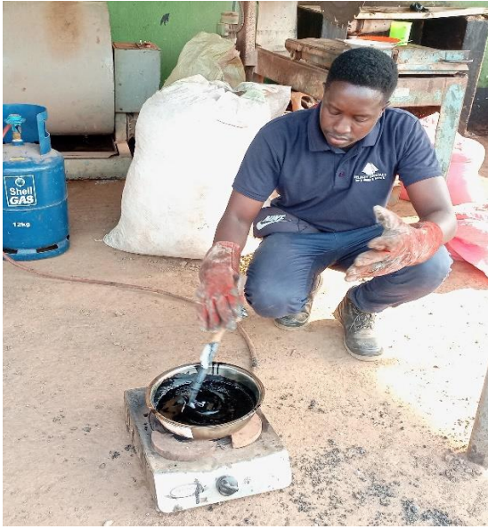
Mixing bitumen and LLDPE homogenously
