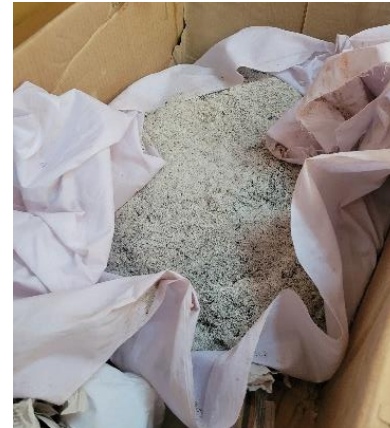
Figure 10: RHA produced at 800 degrees Celsius
