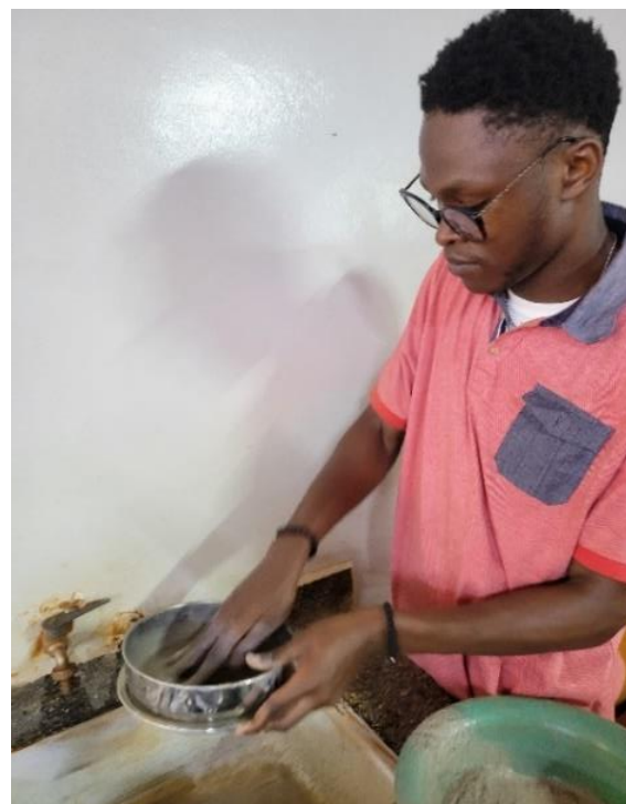
Figure 4: Washing the soil sample (wet sieving)
