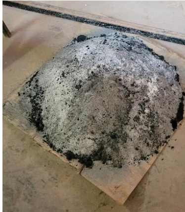
Figure 9: RHA produced at 700 degrees Celsius
