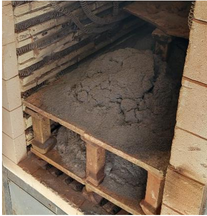
Figure 8: RHA produced at 600 degrees Celsius
