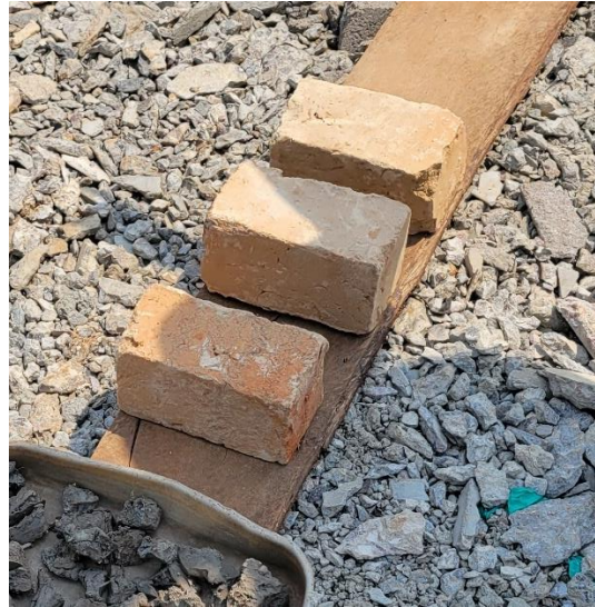
Figure 29: Neat fired clay bricks
