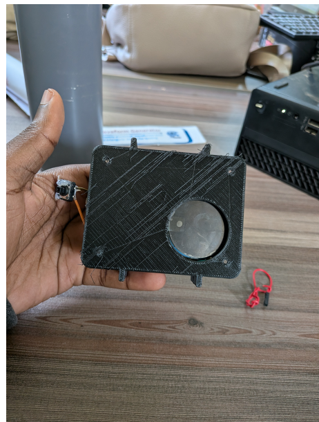
Figure G.2: 3D printed case top part with fitted components
