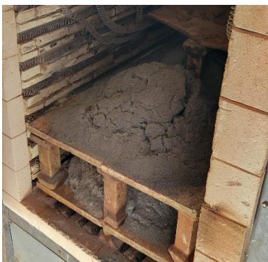
Figure 4: RHA produced at 600 degrees Celsius
