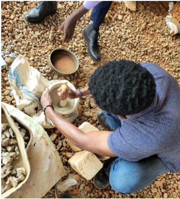
Figure 20 Crushing the soil sample for Atterberg limit tests
