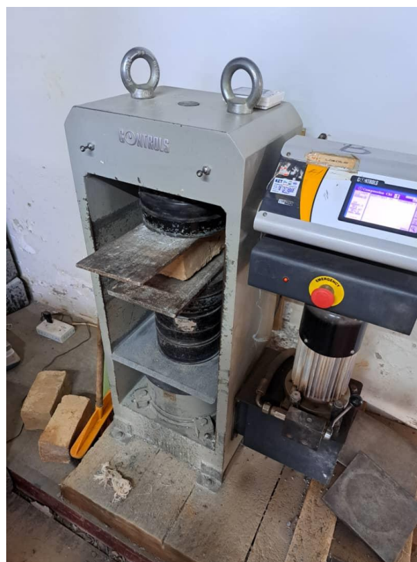
Figure 7: Compressive strength test machine crushing the neat bricks
