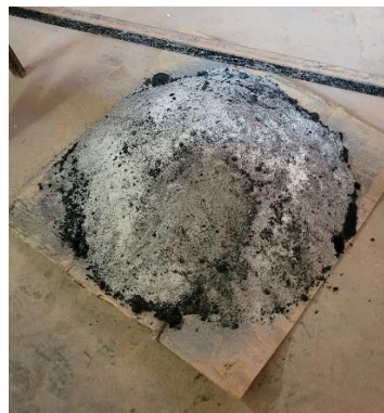
Figure 5: RHA produced at 700 degrees Celsius
