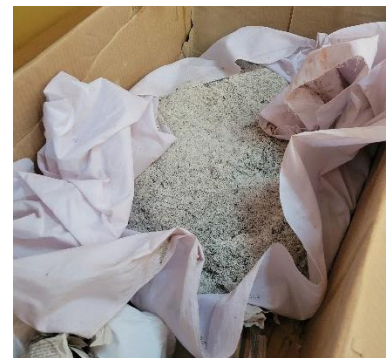
Figure 6: RHA produced at 800 degrees Celsius
