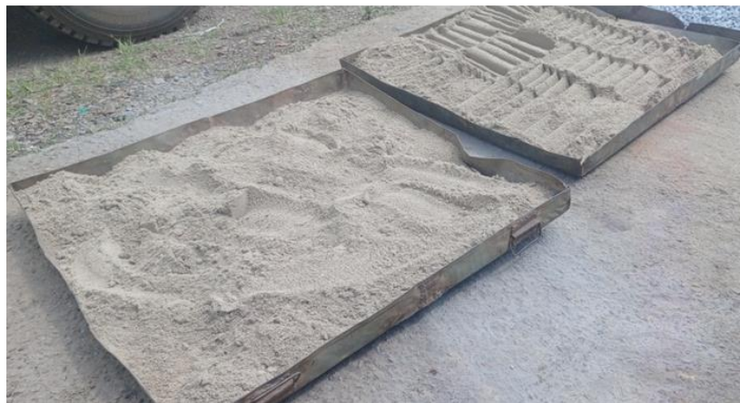
Figure 6 Air drying of the river sand.
