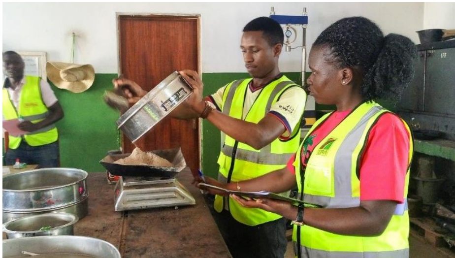
Figure 7 Weighing of the sample retained on the sieves during gradation.
