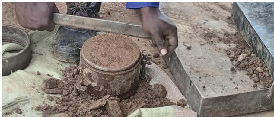
Figure 10 Trimming of the mould after compaction.
