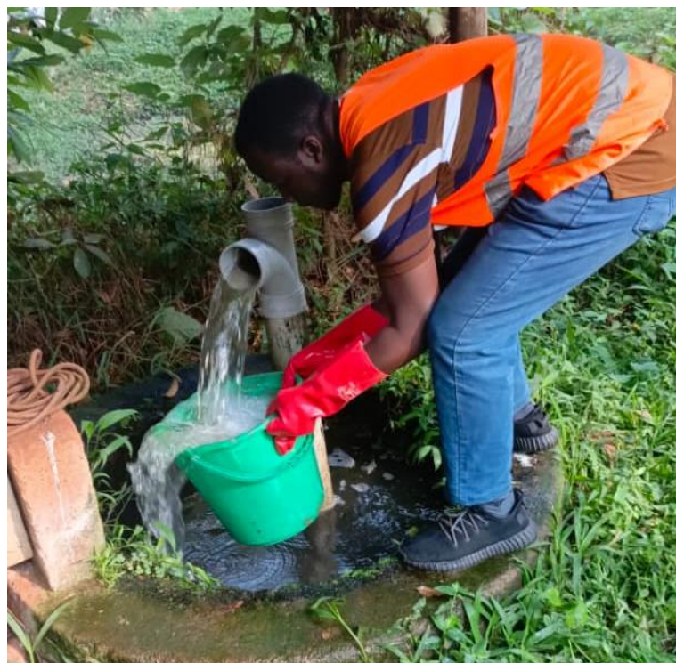
Figure 27: A student collecting effluent in a bucket to determine the flowrate.
