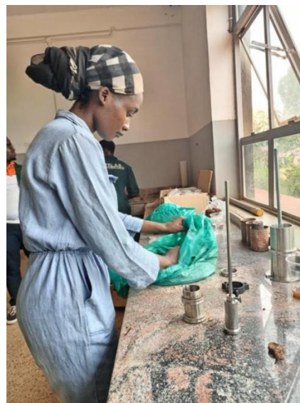
Sample preparation of Triaxial test specimen
