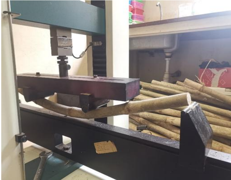
Figure 5: Set up for testing flexural strength, MOE and MOR
