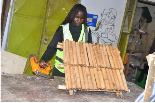
Figure 12: Showing a bamboo roof sample after treating with epoxy resin
