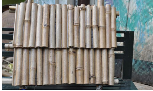
Figure 12: Showing a bamboo roof sample after treating with epoxy resin
