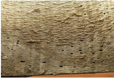
Figure 8: Bamboo eaten by termites
