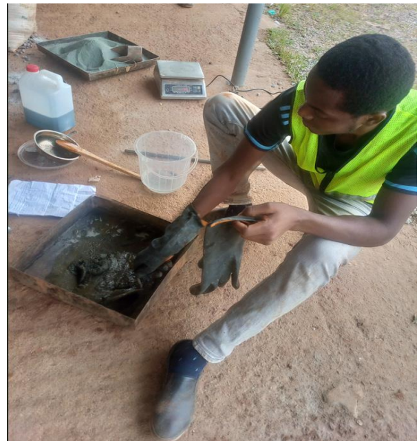
Figure 4: Mixing of granite dust with sodium silicate
