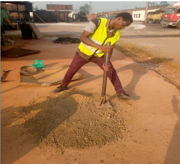
Figure 6: Crashing of the partially hardened clay sample
