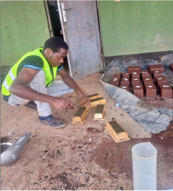
Figure 5: Casting of activated granite dust cubes
