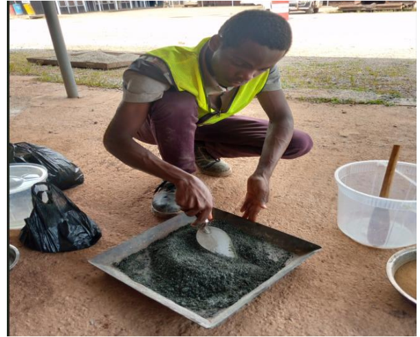
Figure 7: Mixing activated GD with clay for brick making
