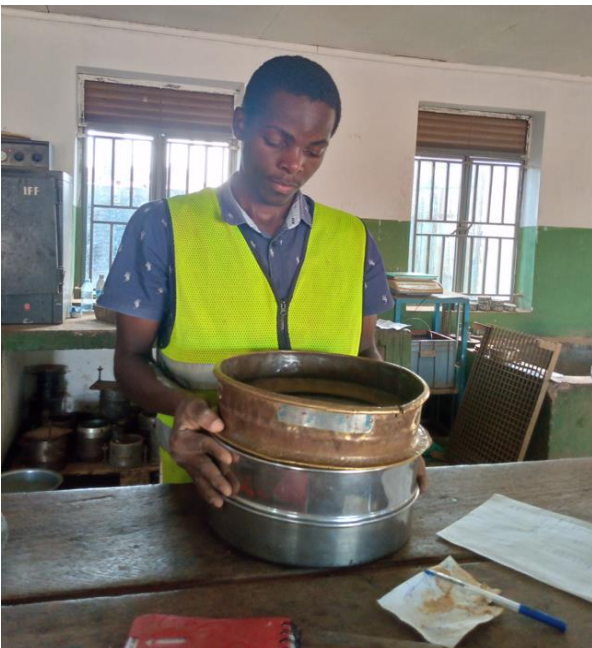
Figure 3: Grading of samples by sieve analysis
