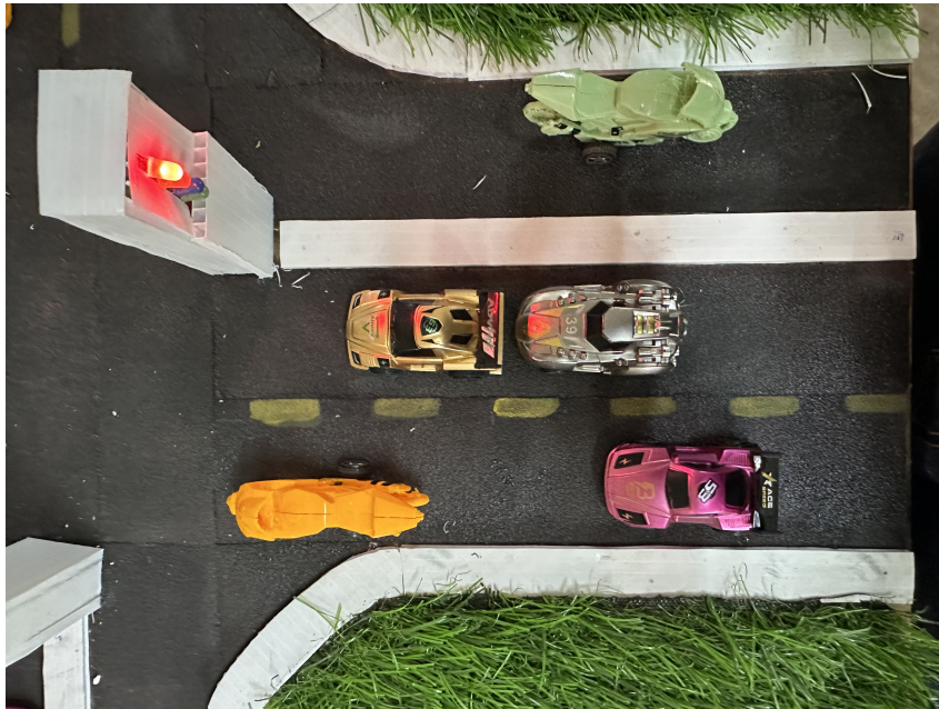
Figure 4.1: Close up of the miniature junction during live inference. The red signal at the top left is being driven by the controller based on YOLO detections.
