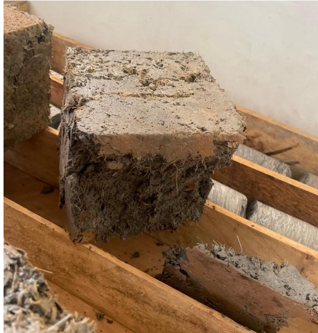
Figure 3.8 Showing the block after crushing
