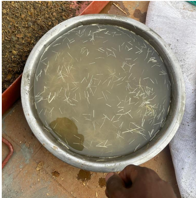
Figure 3.6 Showing the Sisal fibers being soaked before incorporation to the mix
