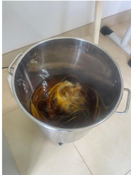
Figure 3.1 Showing Sisal Fibers in the Sodium Hydroxide Solution
