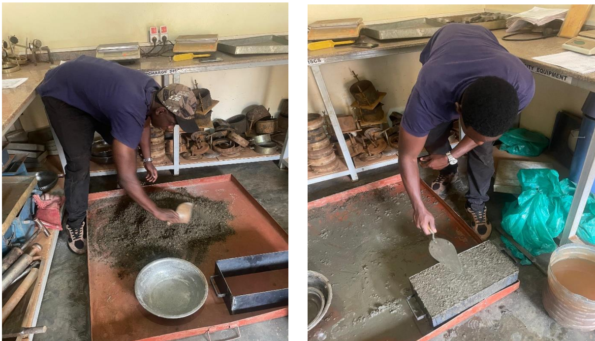
Figure 3.5 Showing the Mixing and Casting of the Woodcrete blocks with sisal fibers
