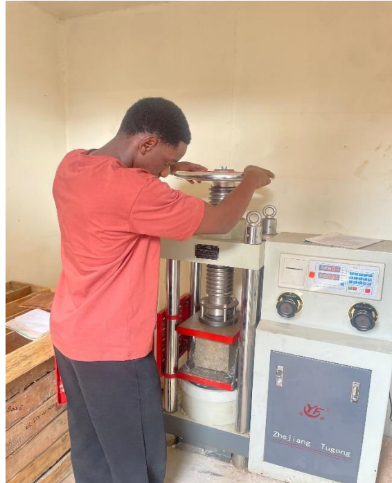
Figure 3.7 Showing the block being prepared for Crushing
