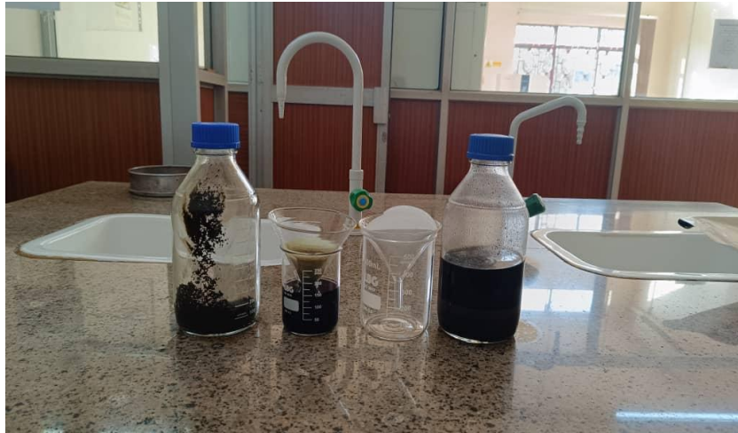
Figure 5: Filtration after trans-esterification to remove any solids
