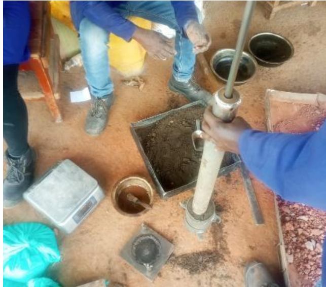
Figure 6: Soil sample for compaction.
