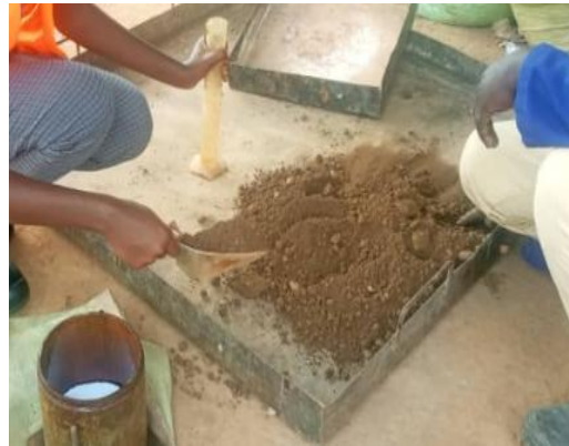
Figure 25: Soil sample for compaction.
