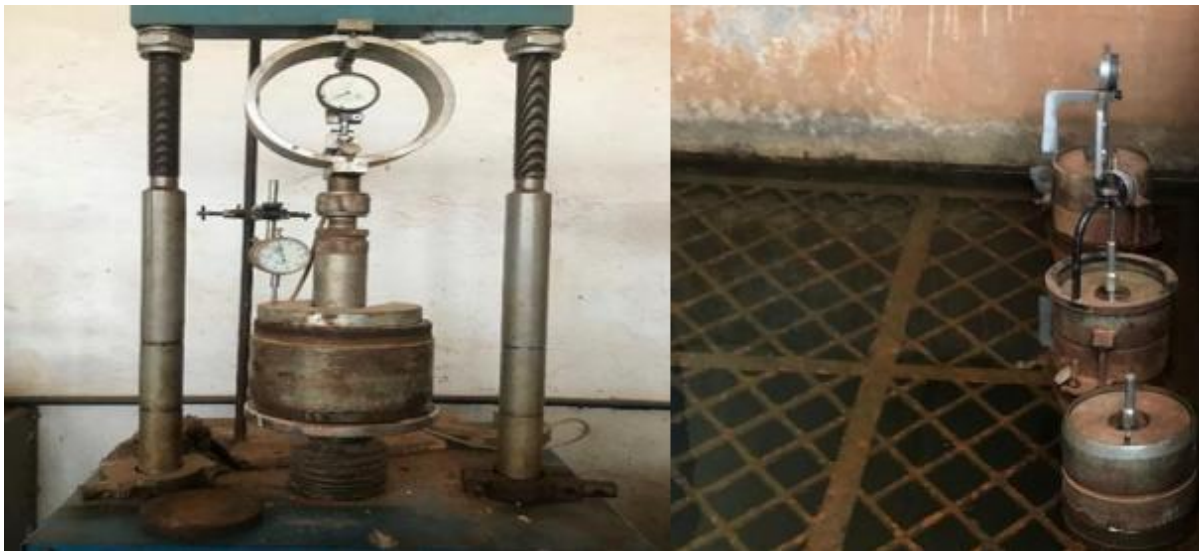
Figure 7: CBR Penetration molds soaking
