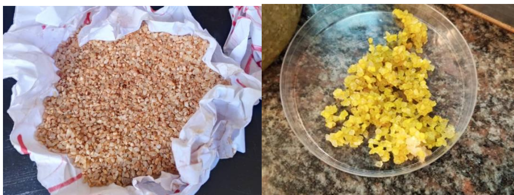
Figure 4: Coated quartz sand before and after oven drying
