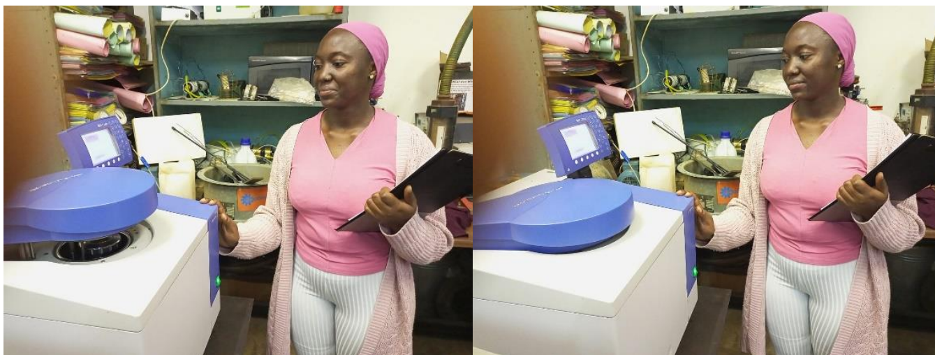
Figure 34: Inserting the Bomb into the calorimeter and starting the test.
