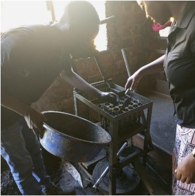
Figure 38: Injecting the mixture into the briquette machine
