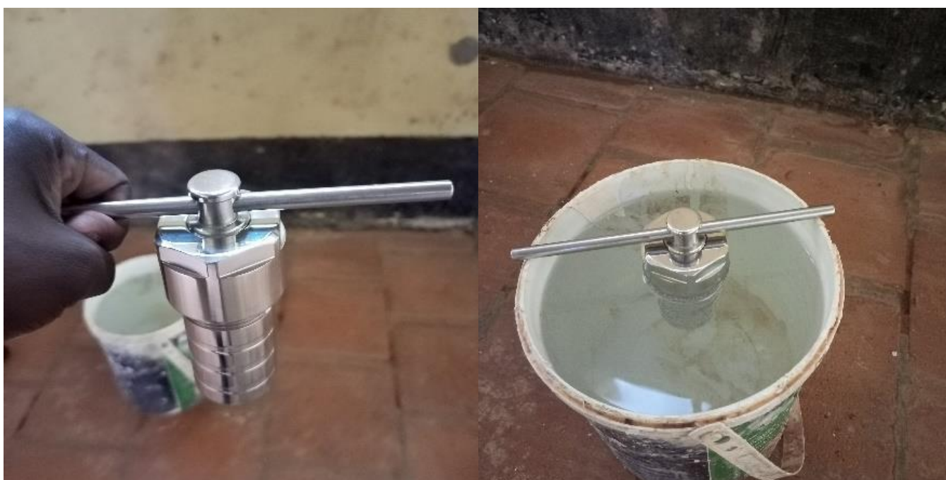
Figure 30: Rapidly cooling the reactor with water
