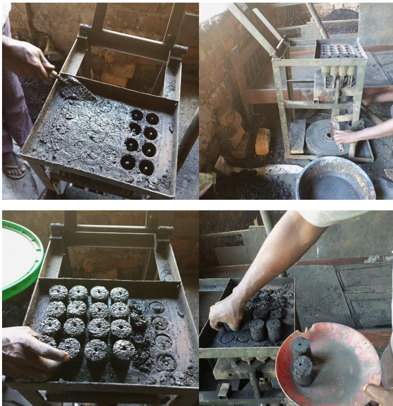
Figure 40: Extruding the briquettes from the briquetting machine.
