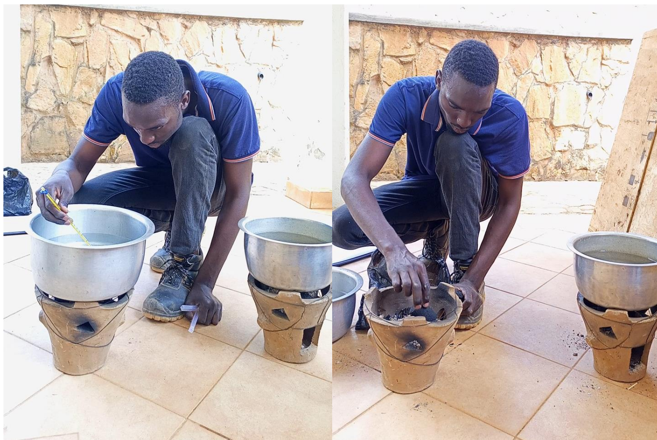
Figure 46: Water boiling test
