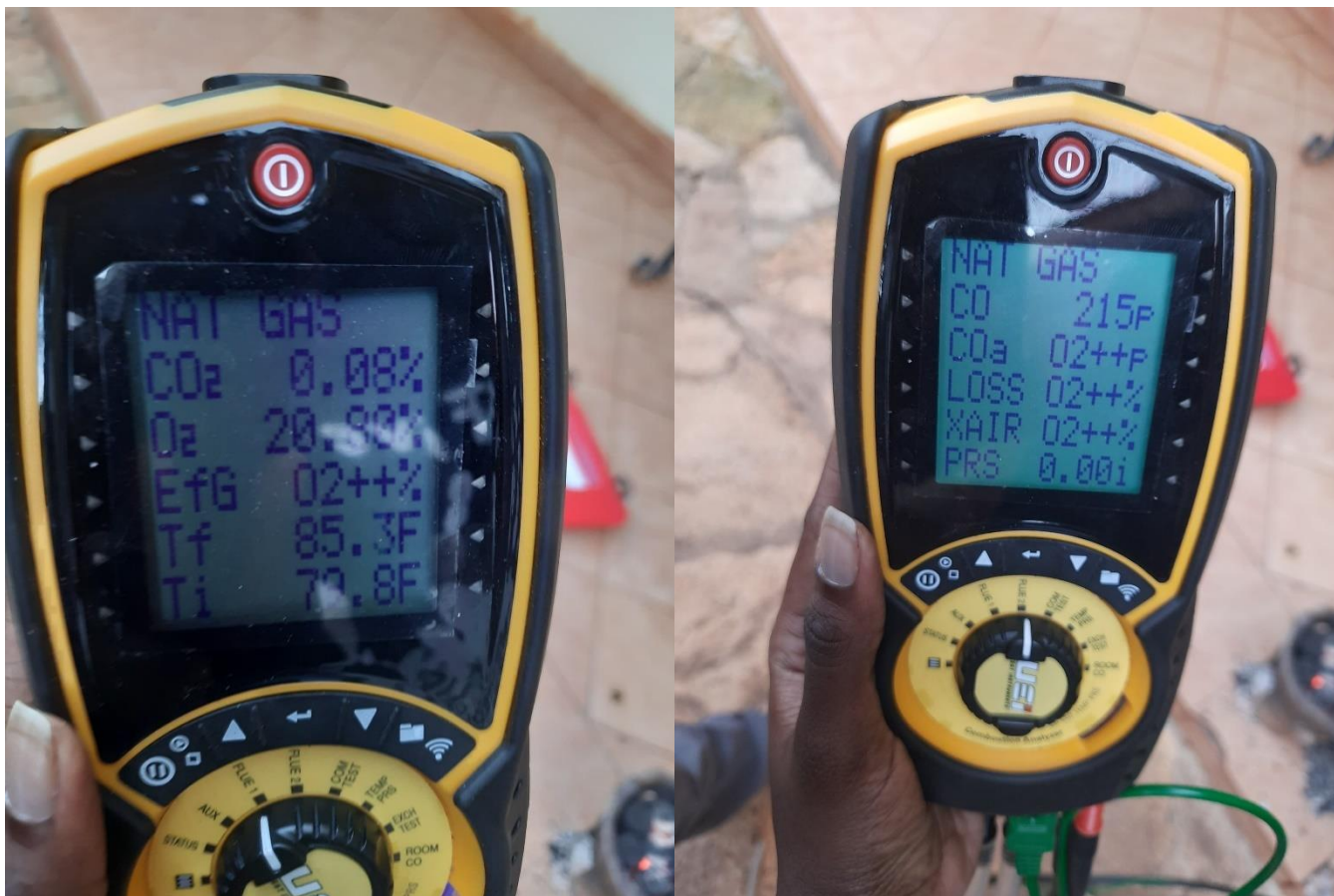
Figure 44: Flue gas testing
