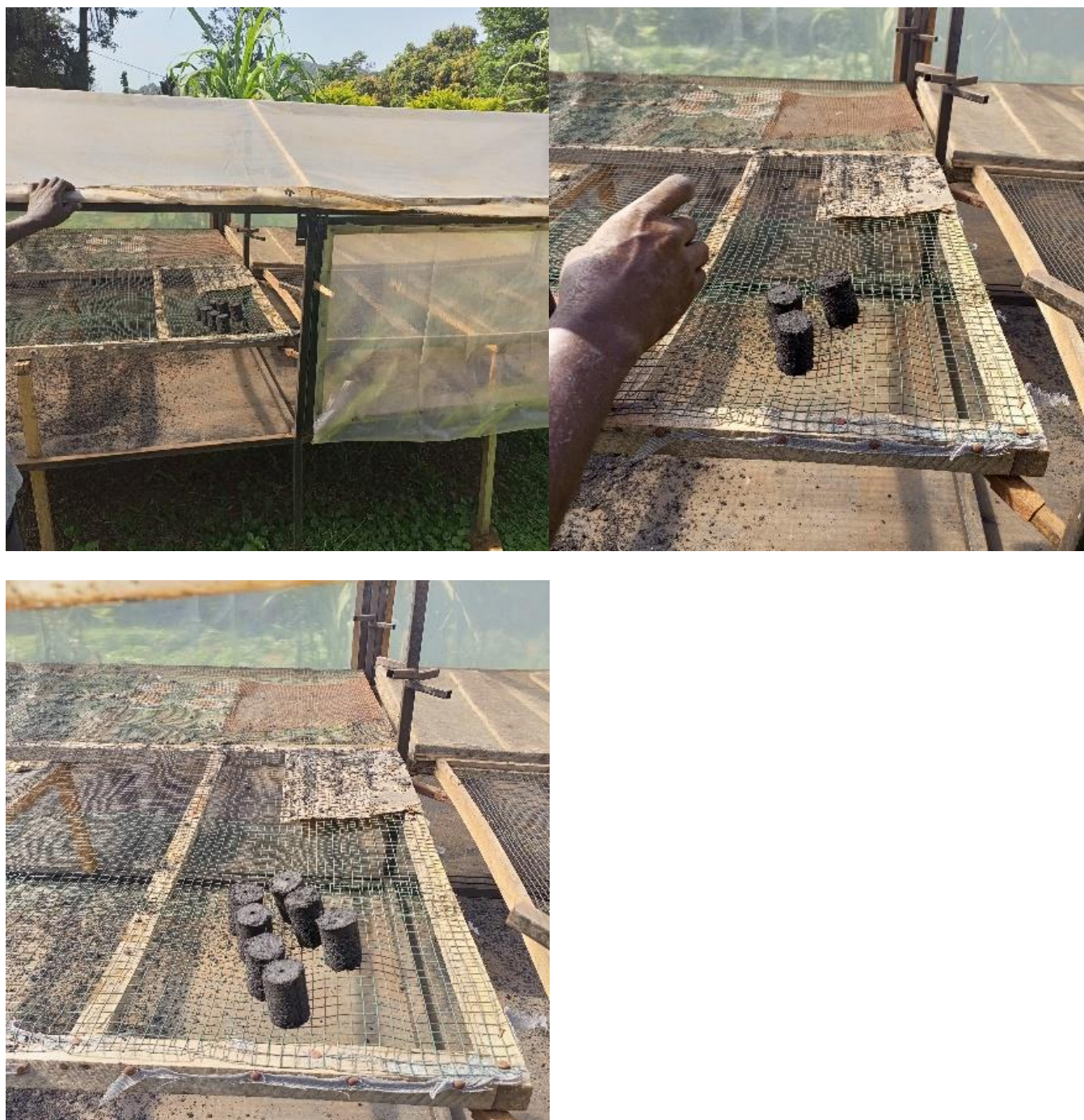
Figure 41: Drying the Briquettes made in an air dryer
