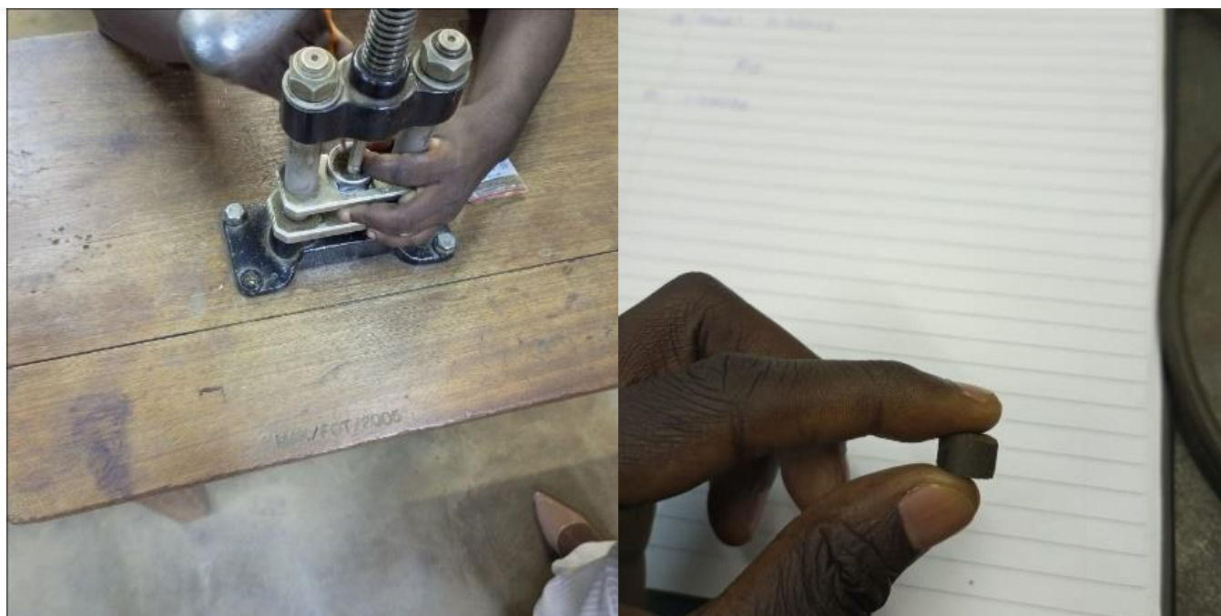
Figure 31: Briquetting the sample before testing.
