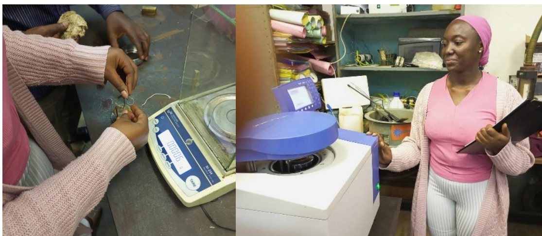
Figure 6: Using the bomb Calorimeter to determine the calorific value.
