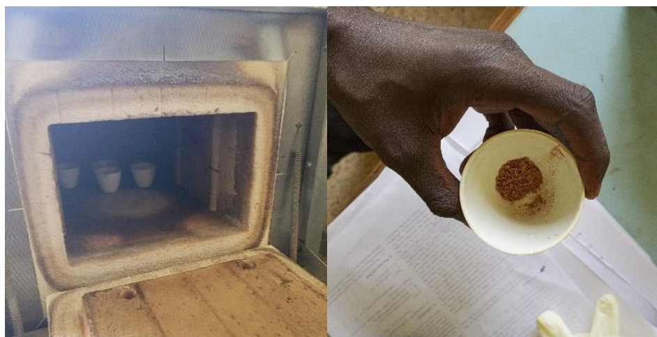
Figure 4: Ash Content Test
