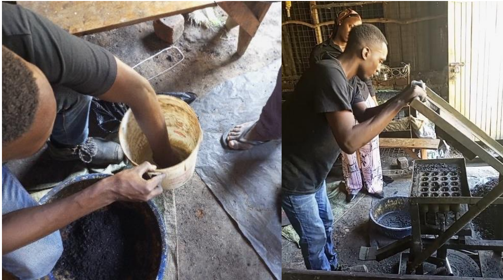
Figure 7: Sample preparation and Compaction
