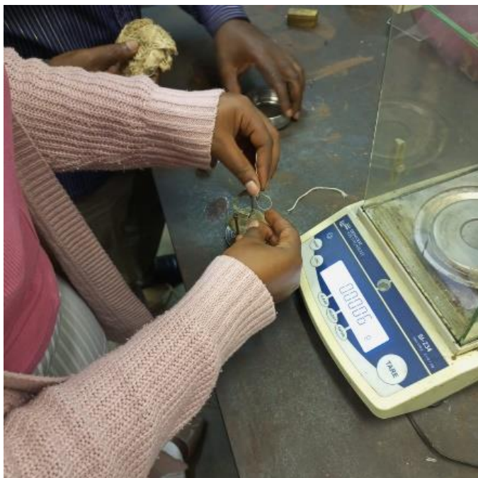
Figure 33: Loading the sample into the bomb
