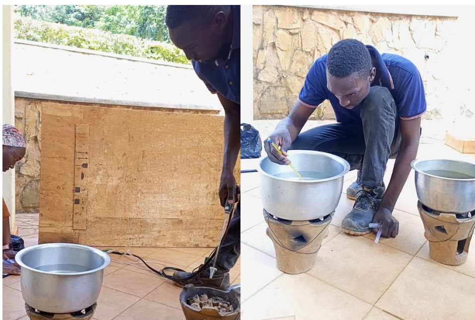
Figure 9: Flue gas emission test and measuring the change in water temperature.
