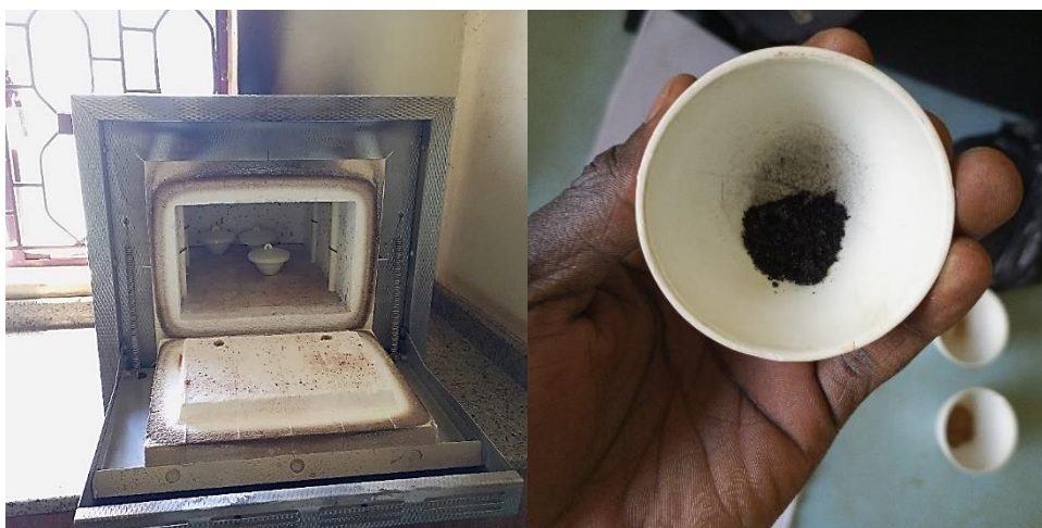
Figure 3: Volatile matter test
