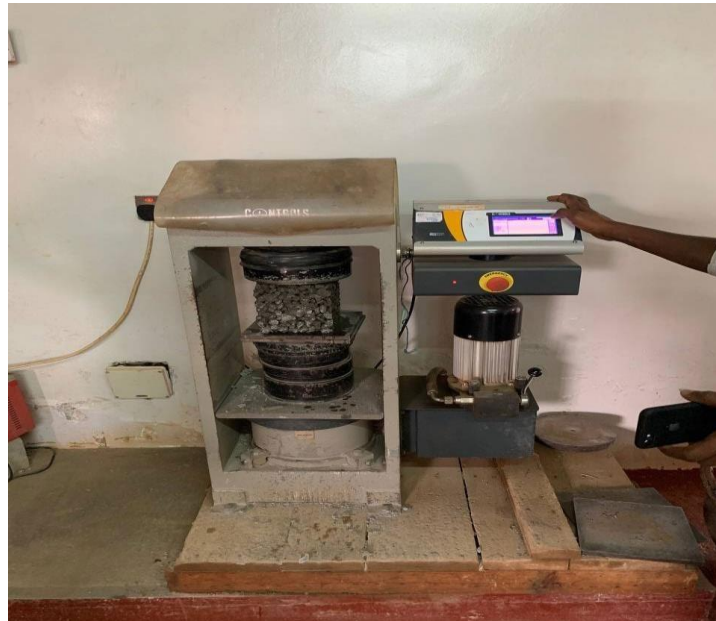
Figure 7: Experimental setup for compressive strength test
