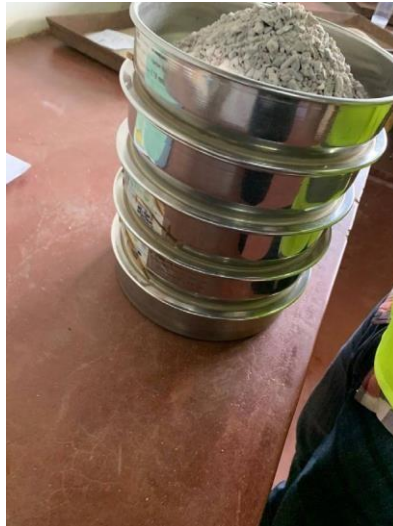
Figure 6: Experimental setup for the particle size distribution test
