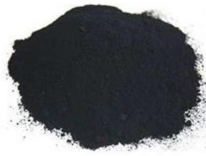
Figure 6-7: Black char form pyrolysis
