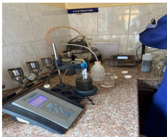
Figure 8 Determination of pH and electrical conductivity
