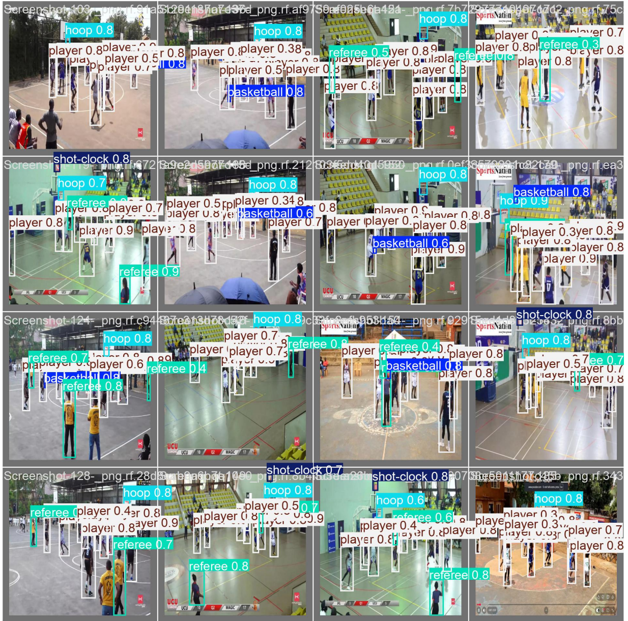
Figure 4.5: Ball Detector validation output showing successful identification of the basketball in a high-clutter game scenario.
