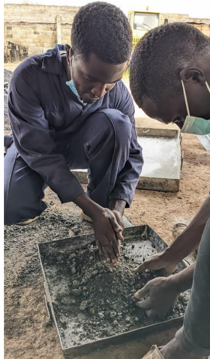
Figure 3: Mixing of 6% hydrated lime and 94% dry weight of expansive soil. Source (Manana, 2024).
