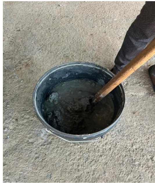
Figure 15: activating the waste glass powder with NaOH
