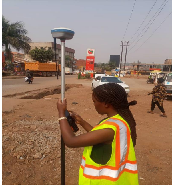
Figure 10: Topographic survey with the RTK GPS
