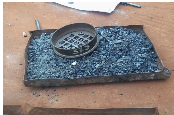
Figure 23: Crushed steel slag
