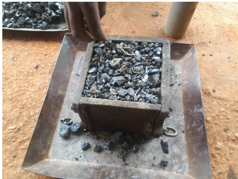
Figure 6: Mould filled with steel slag.
