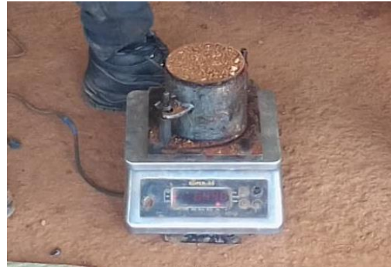
Figure 19: Weighing of proctor sample mould after compaction
