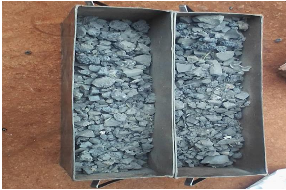
Figure 24: Riffing of steel slag process.
