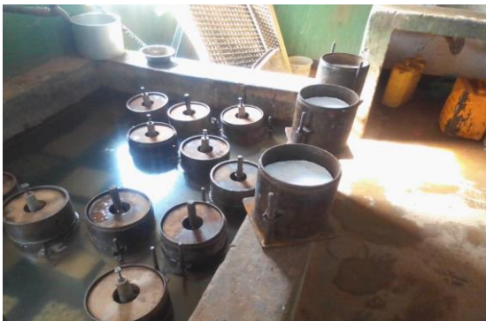
Figure 20: CBR samples ready for soaking
