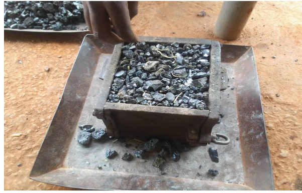
Figure 25: Steel slag bulk density test
