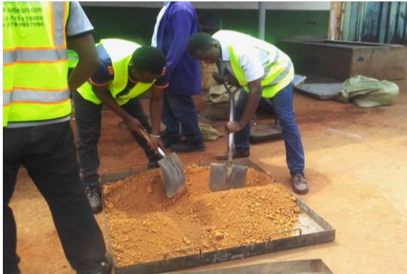
Figure 18: Quartering of neat sample for testing
