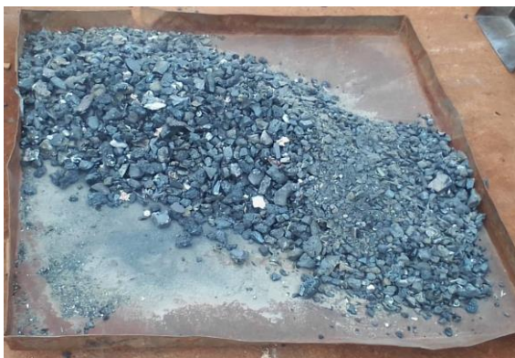
Figure 2: Crushed steel slag material.
