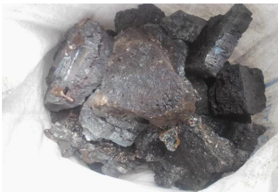
Figure 22: Steel slag from Roofings steel melting plant waste
