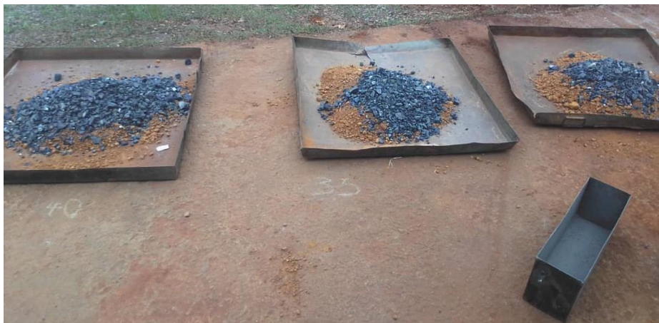
Figure 7: Varying percentages of steel slag added to laterite soil.
