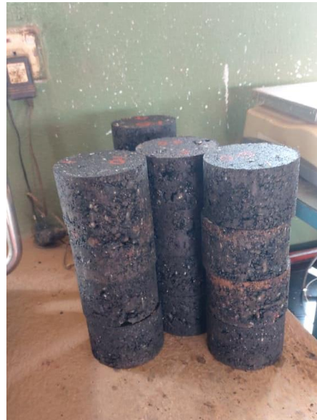
Figure 9: Shows compacted asphalt
