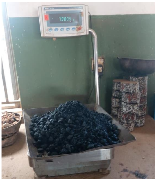
Figure 8: Shows an asphalt sample Marshalls
