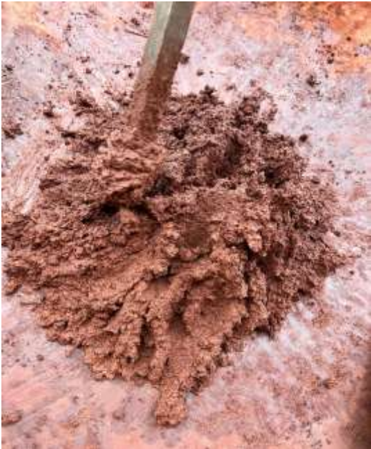
Figure 4: Mortar ready for molding
