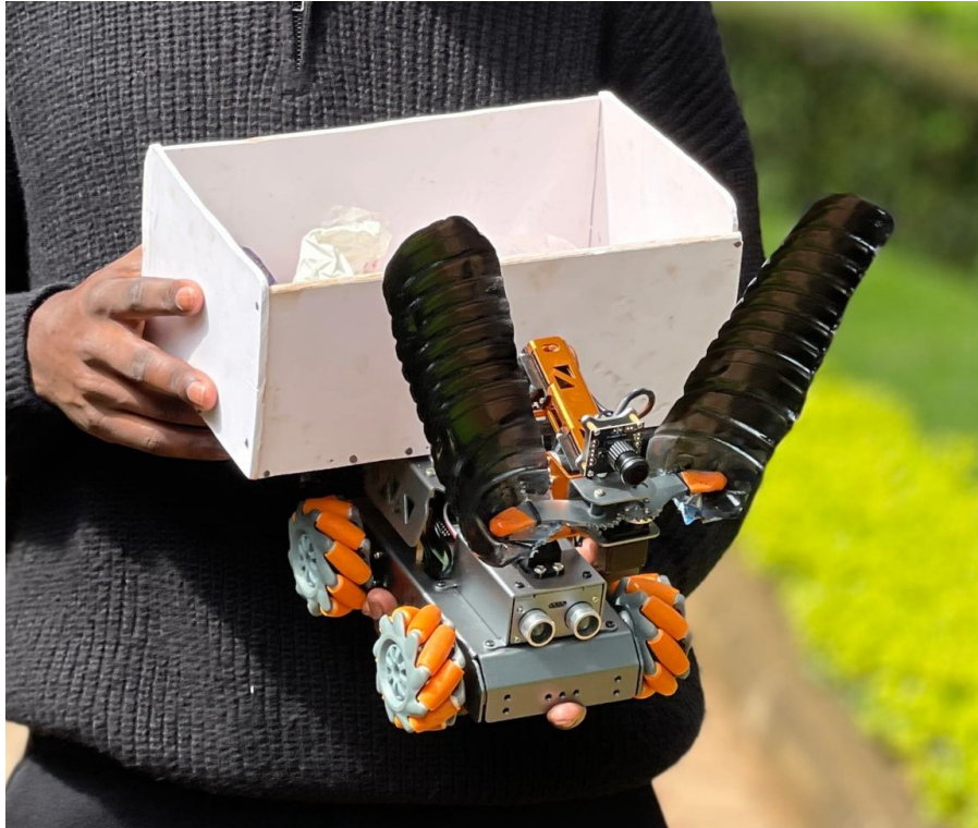
Figure D.2: ECO-BOT with onboard waste collection bin mounted at the rear for storing collected litter
