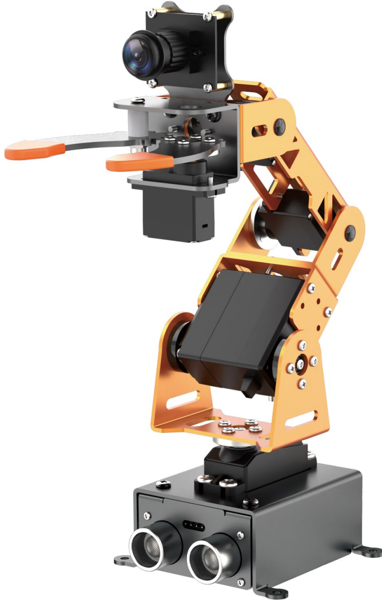
Figure 3.4: 5-DOF robotic arm module with integrated camera and gripper used for waste detection and collection
