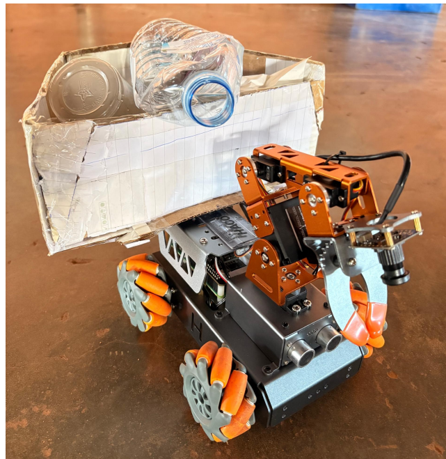
Figure D.5: ECO-BOT interacting with waste during testing, demonstrating positioning of the robotic arm near the collection bin
