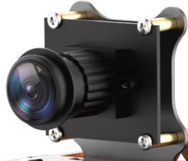
Figure 3.5: Front-mounted camera module used for real-time litter detection in the ECO-BOT system
