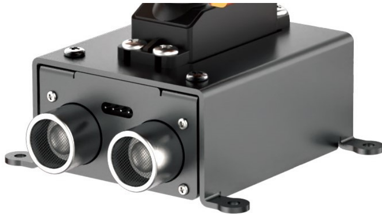
Figure 3.6: Ultrasonic sensor used for obstacle detection and distance measurement during navigation
