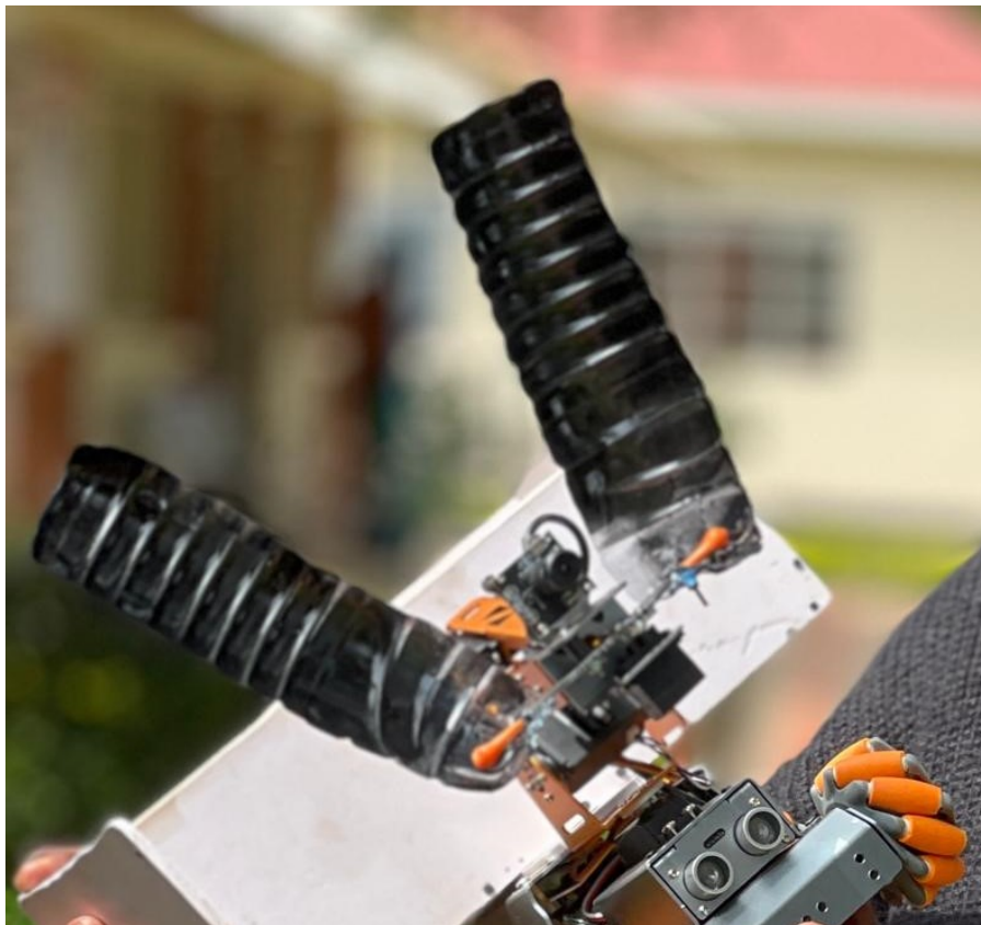
Figure D.6: Modified scooper-based end-effector used for collecting lightweight waste materials such as plastic bottles and polythene bags
