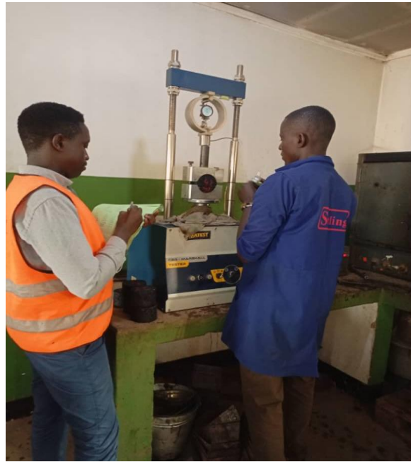
Figure 30 Marshal Stability and Flow test
