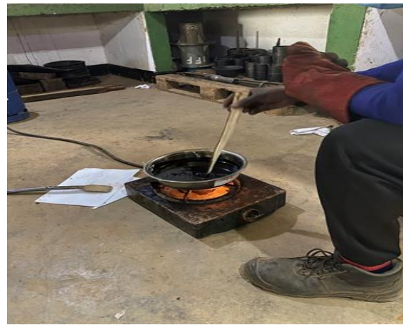
Figure 26 Mixing LLDPE with bitumen
