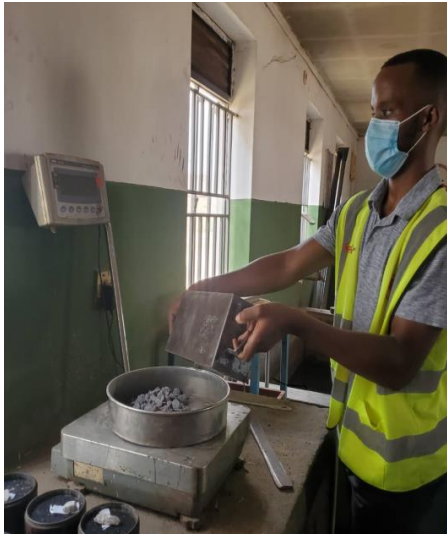
Figure 5: Weighing of aggregates
