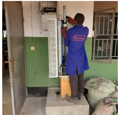
Figure 8: Compaction of Marshall cores
