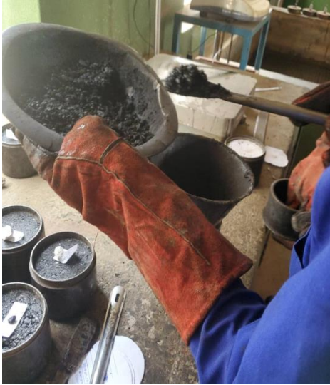
Figure 9: Placing of asphalt in moulds
