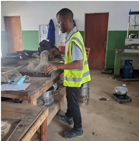
Figure 7: Mixing of AC 14 with filler
