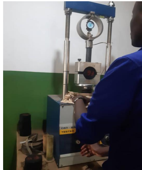
Figure 12: Marshall and ITS Testing
