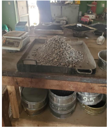
Figure 6: Final mix by mass of mix design
