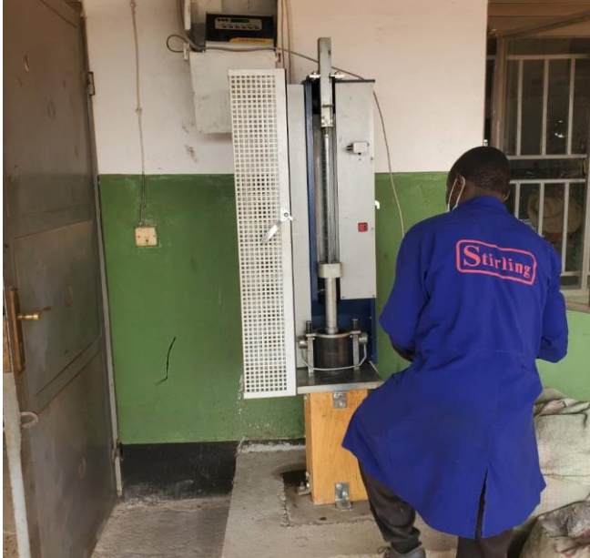
Compaction of Marshall Cores
