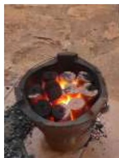
Figure 6: ignited briquettes in the stove
