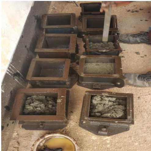
Casting of concrete cubes
