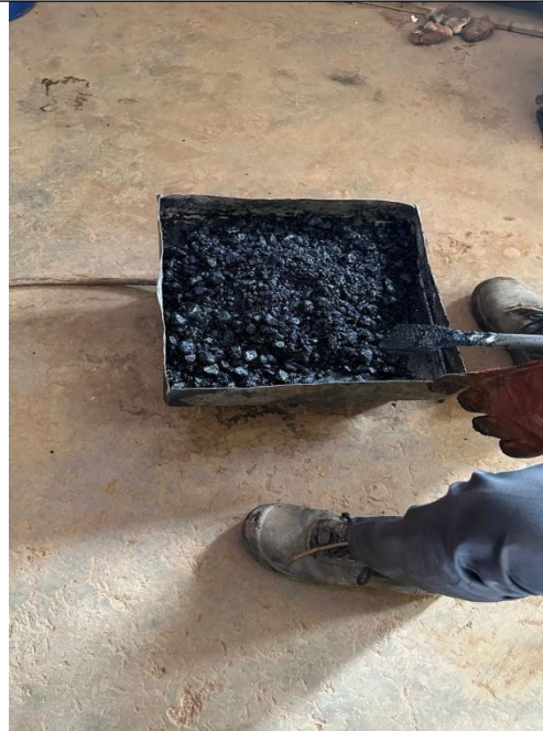
Image 4 The Marshall sample mixed homogeneously
