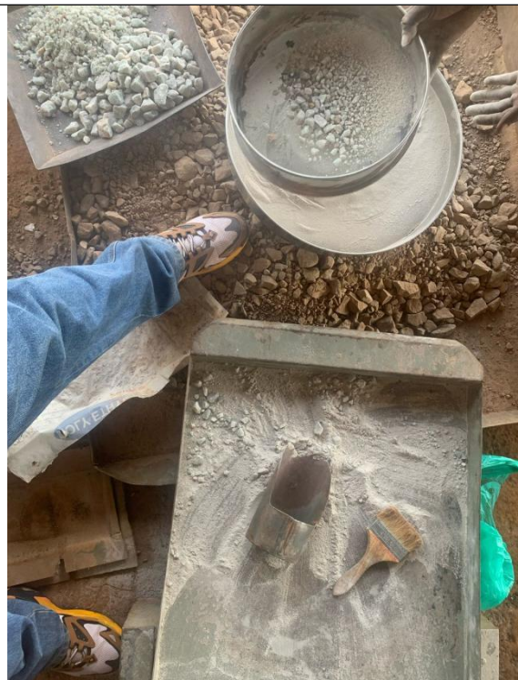
Image 2 Quartzite filler sieving
