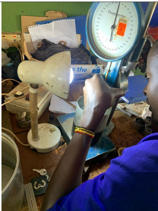
Image 5 Bitumen Penetration test
