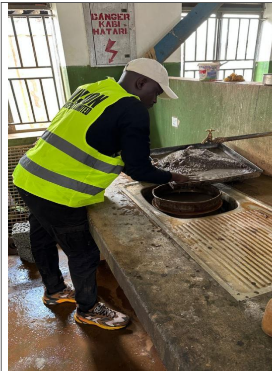
Image 1 Wet sieving for grading
