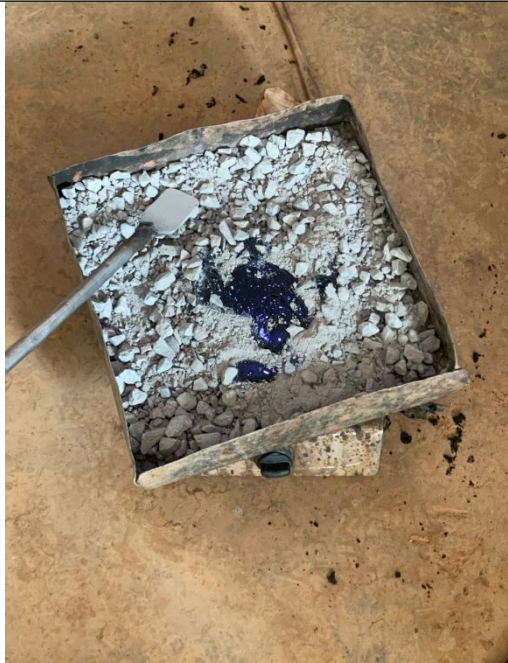
Image 3 Marshall Mix preparation
