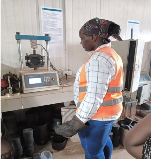
Stability and flow test
