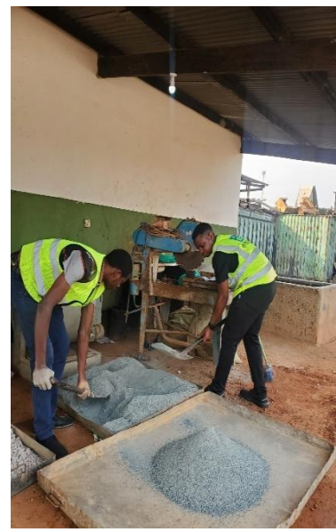
Figure 2: Sampling of the granite dust for cube
