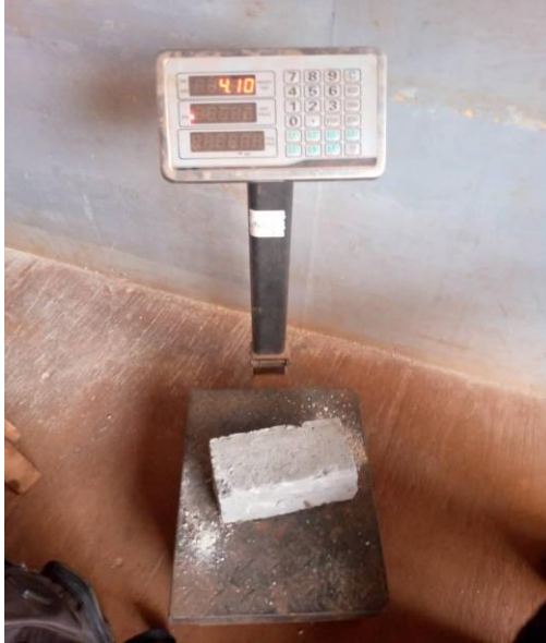
Figure 11: Determining the weight of the final brick product
