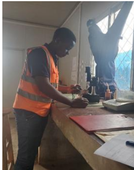
Figure 6: Liquid limit test
