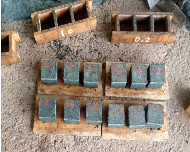
Figure 7: The geopolymer cubes after 28 days of air drying
