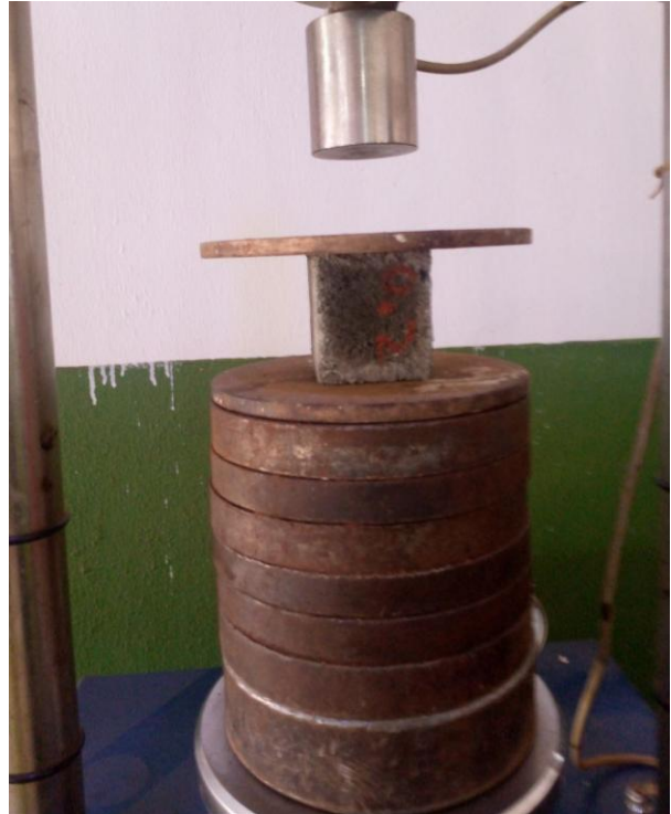
Figure 8: Compressive strength test on the geopolymer cubes
