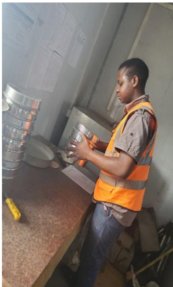
Figure 4: Particle size distribution test
