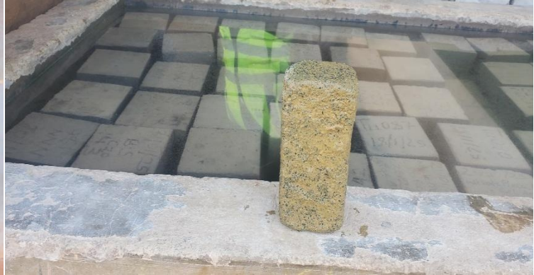
Figure 12: Final brick product after the water absorption capacity test
