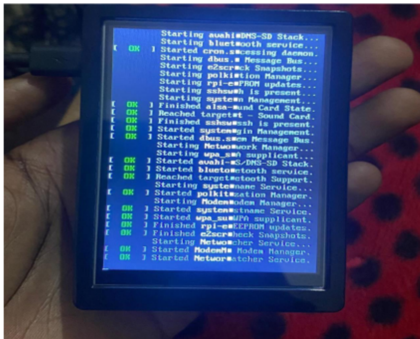
Figure H.6: Raspberry Pi Device – Boot Screen: System initialization and runtime execution.
