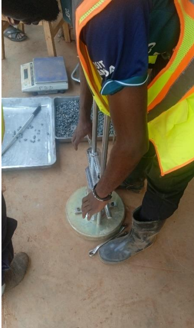
Figure 5: Aggregate impact value test
