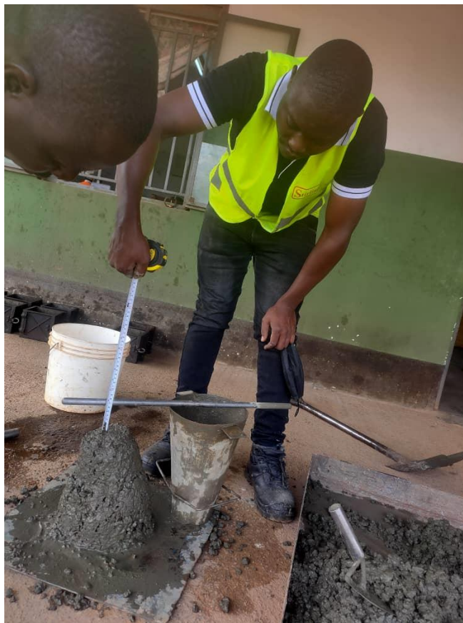
Figure 6 : Slump test for concrete
