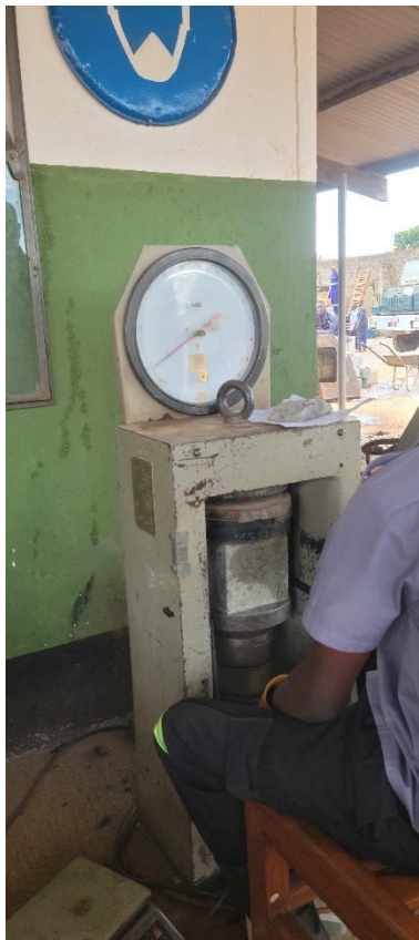
Figure 7: Compressive strength test for concrete cubes
