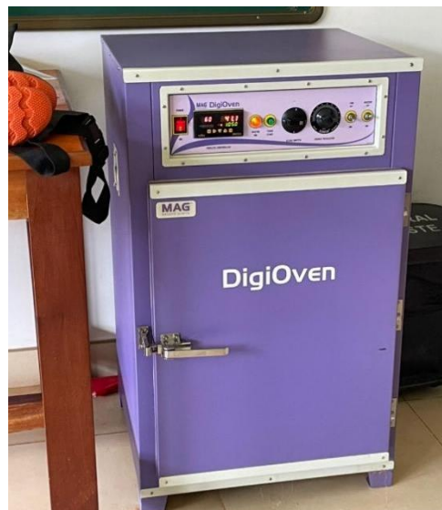
Figure 7: An oven drier used for drying specimen
