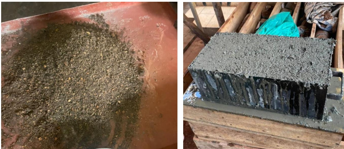
Figure 5: Mixing and casting of a block unit
