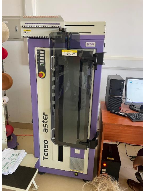
Figure 3: Tensometer machine for tensile strength testing
