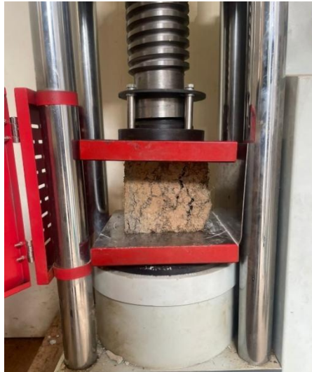
Figure 6: Block under a UTM for compressive test
