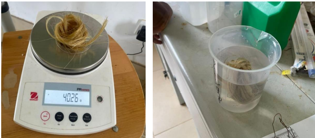
Figure 4: Testing for density of the sisal fibers
